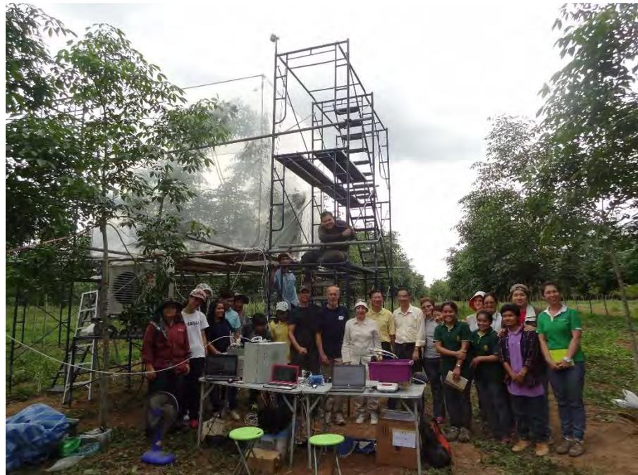
**Figure 6** Overview of the large closed-chamber designed to field measure photosynthesis of whole tree crowns and pulse label trees with  $^{13}\text{CO}_2$ , installed on a rubber tree.
