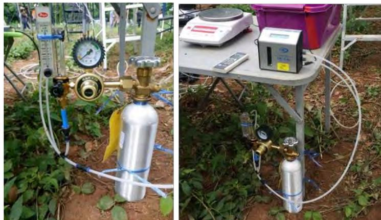
**Figure 11**  $^{13}\text{CO}_2$  from gas cylinder was constantly injected into the labelling chamber using a primary air flow meter at a rate adjusted to balance the estimated net rate of  $\text{CO}_2$  consumption by crown photosynthesis.
