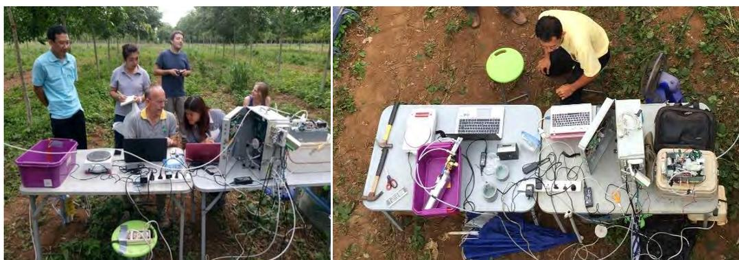
**Figure 9** The control system and data logger to measure tree crown  $\text{CO}_2$  exchange rates and pulse-label trees with  $^{13}\text{CO}_2$ .
