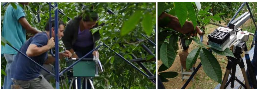
**Figure 13** Leaf photosynthesis of rubber tree by using a portable gas exchange analyzer (Li6400XT; LI-COR Lincoln, NE, USA).
