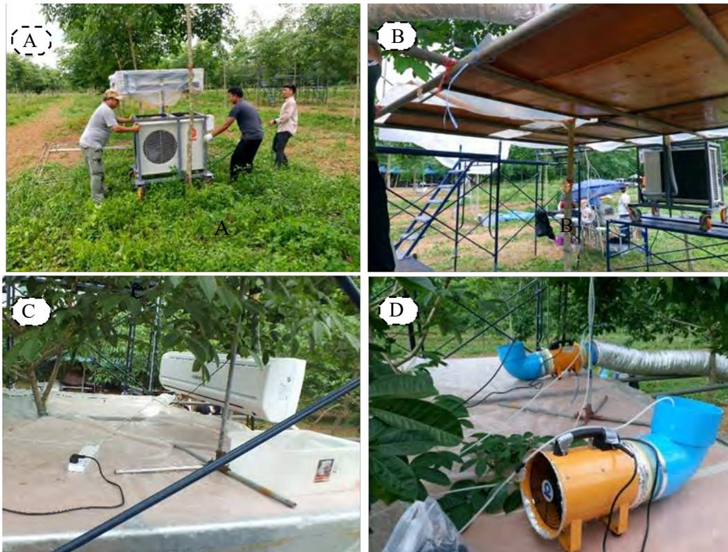
**Figure 10** (A–C) Air cooling ensured by air conditioning unit, (B) the compressor part was placed outside chamber but (C) the cooling part and (D) air mixing using two air blowers were placed inside chamber.
