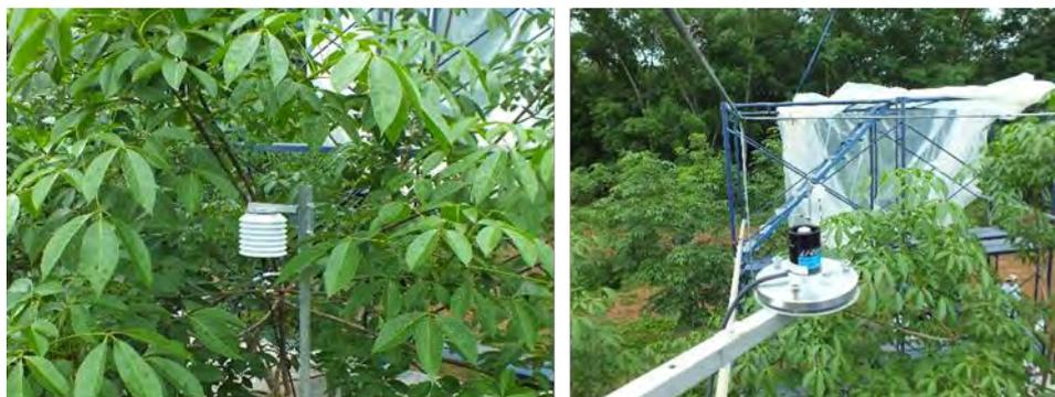
**Figure 12** Sensors measuring air temperature and humidity below canopy (left), and photosynthetic photon flux density above canopy (right).
